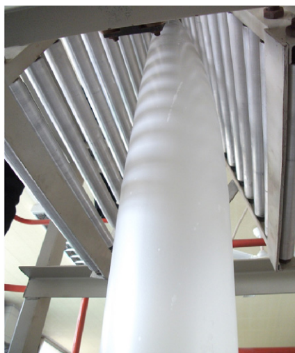
Fig. 1. Continuous and stable film blowing of starch–nanoclay composites.
